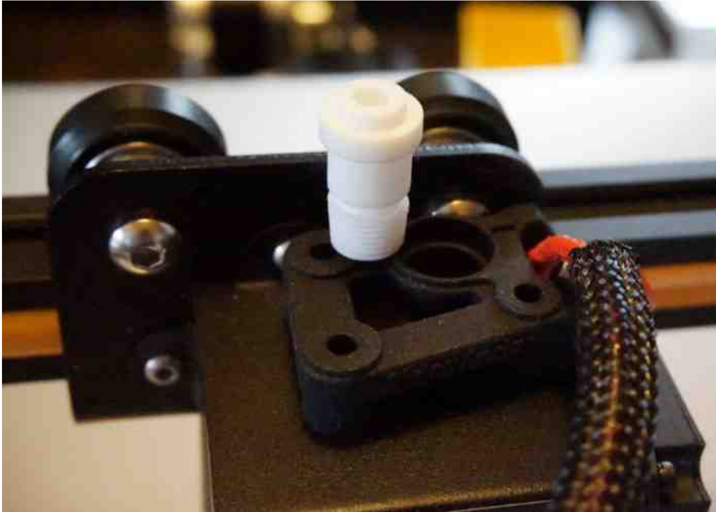
Fig. 3: Pull the block forward until the mount screw will slide down into the hot end.
