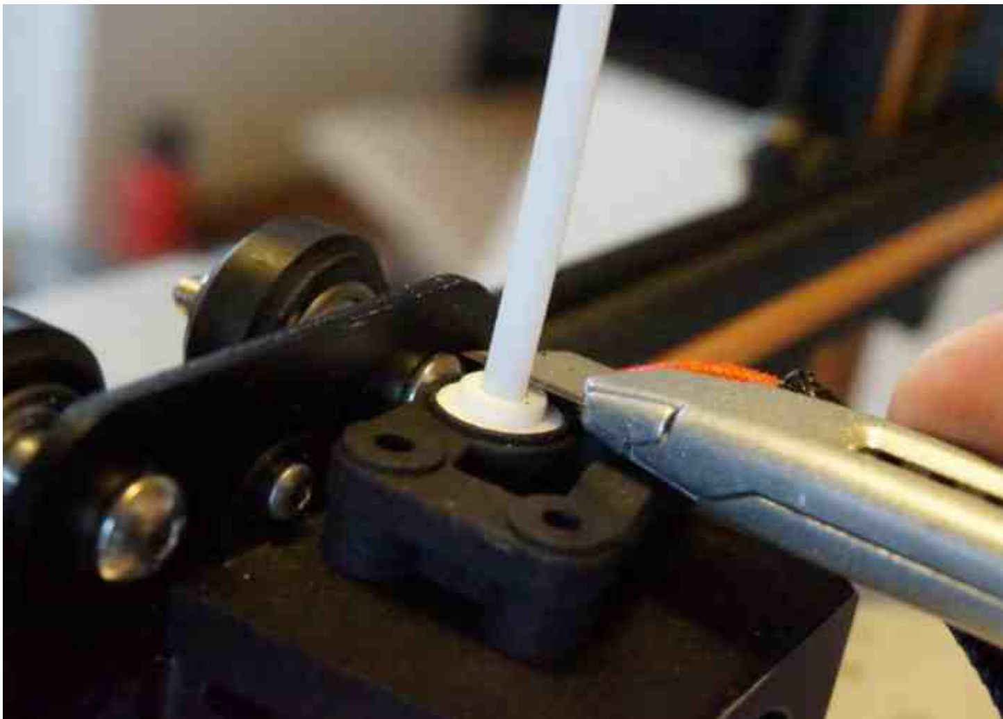
Fig. 5: Slice off the PTFE tube at the top Flush with the top of the mounting screw.
