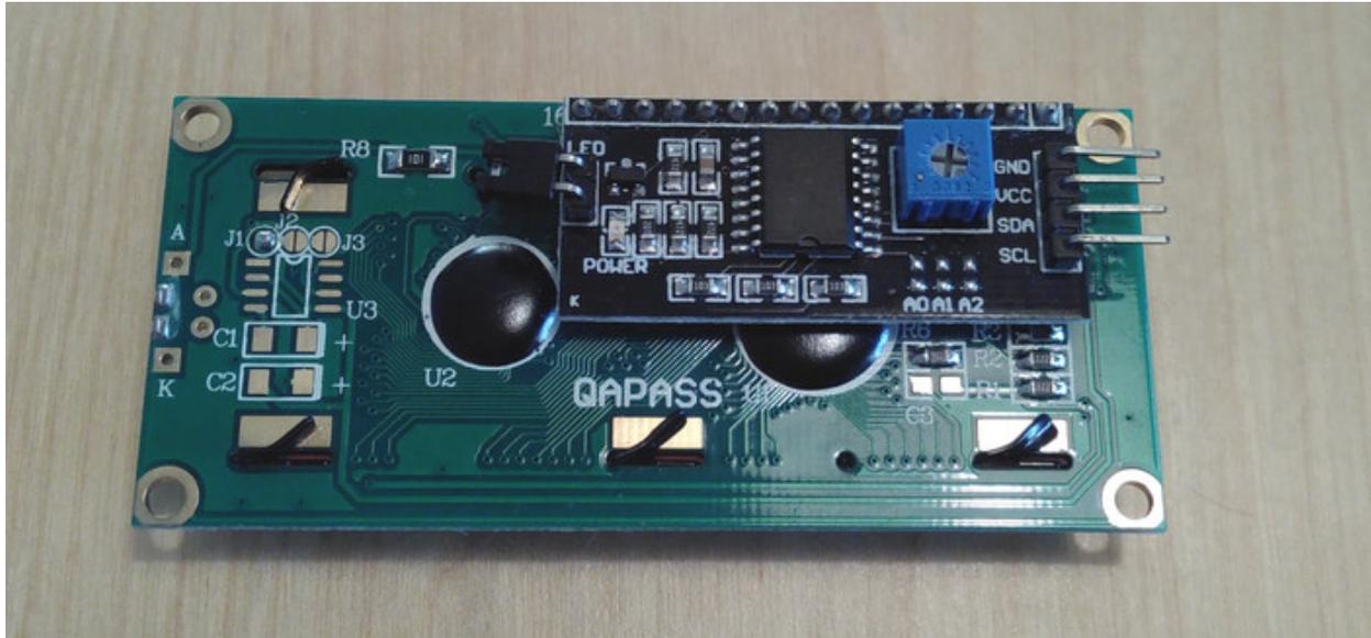
The board on this photo has a PCF8574 port expander chip on it. There are also boards with other chips, e.g. the Adafruit I<sup>2</sup>C/SPI LCD Backpack which uses an MCP23008 port expander.
