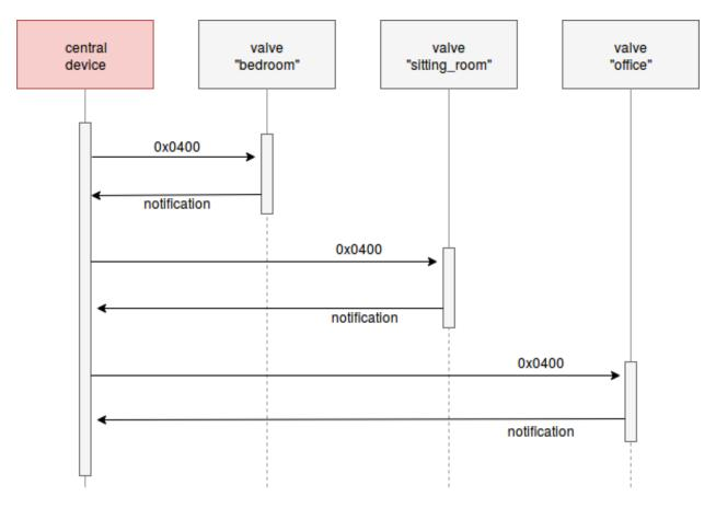
Fig. 31: Sequence Diagram of auto\_mode.sh
