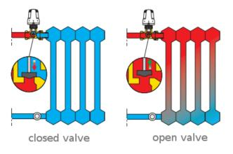
Fig. 2: Operating scheme of a classic valve<sup>1</sup>
