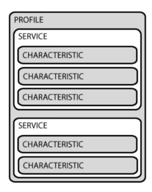
Fig. 8: Hierarchy of profiles, services and characteristics<sup>5</sup>
