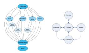
Fig. 9: BR/EDR States<sup>12</sup> (left) // BLE States<sup>13</sup> (right)
