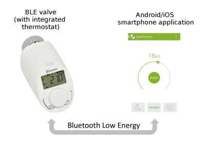
Fig. 3: Electronic BLE valve
