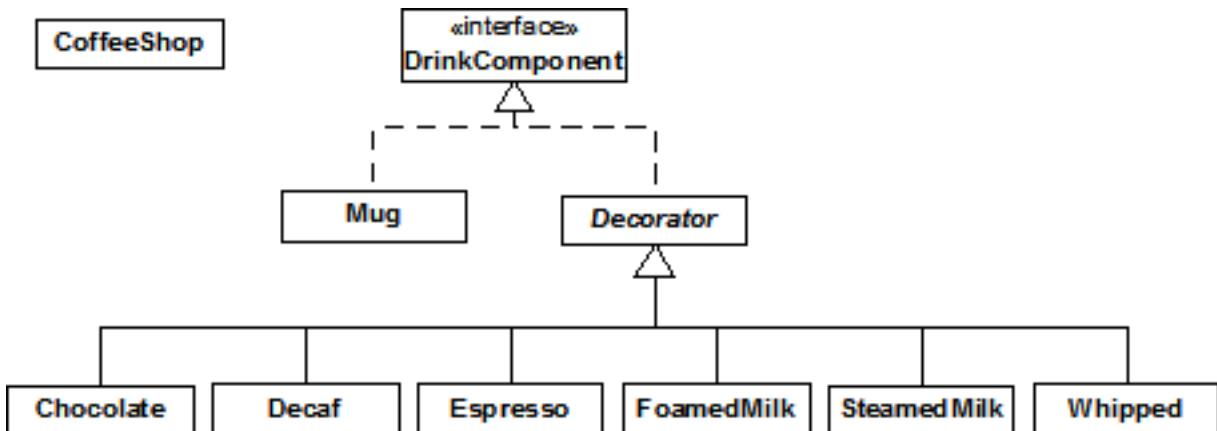
Methods invoked on the **Decorator** can in turn invoke methods in the component, and can of course perform processing before or after the invocation.
