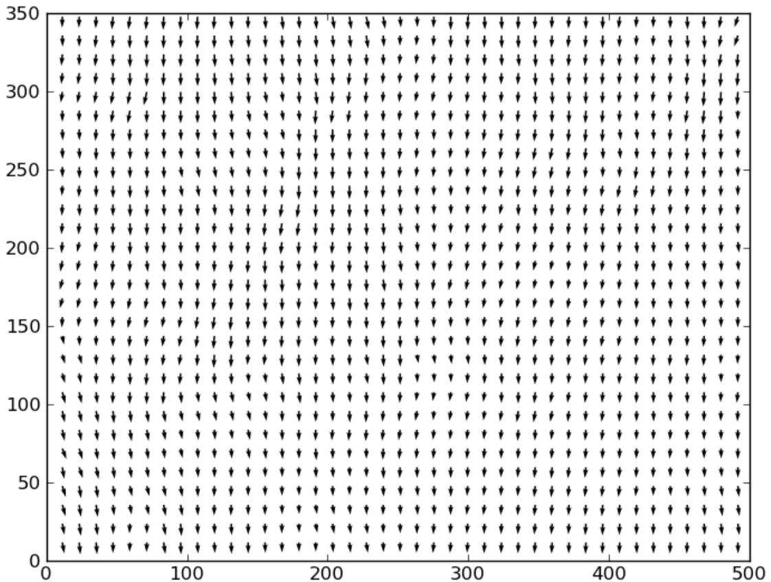
The last step is to apply an uniform scaling to the flow field to get dimensional units. We use the function `openpiv.scaling.uniform()` providing the `scaling_factor` value, in pixels per meters if we want position and velocities in meters and meters/seconds or in pixels per millimeters if we want positions and velocities in millimeters and millimeters/seconds, respectively.
