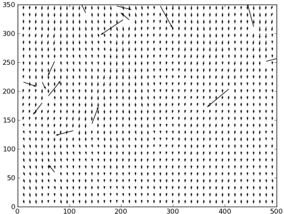
Several outliers vectors can be observed as a result of the small interrogation window size and we need to apply a validation scheme. Since we have information about the signal to noise ratio of the cross-correlation function we can apply a well know filtering scheme, classifying a vector as an outlier if its signal to noise ratio exceeds a certain threshold. To accomplish this task we use the function:
