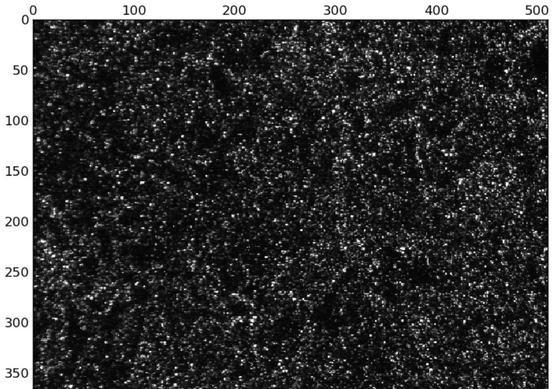
In this example we are going to use the function `openpiv.process.extended_search_area_piv()` to process the image pair::
