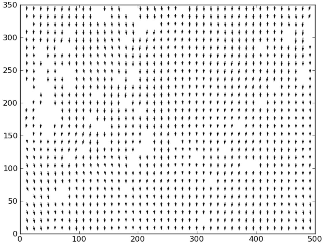
The final step is to replace the missing vector. This is done with the function `openpiv.filters.replace_outliers()`, which implements an iterative image inpainting algorithm with a specified kernel. We pass to this function the two velocity components arrays, a method type `localmean`, the number of passes and the size of the kernel.:
