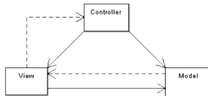
Fig. 1.2: Model-View-Controller diagram
