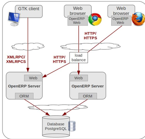
Fig. 1.1: OpenERP 6.1 architecture for embedded web deployment
