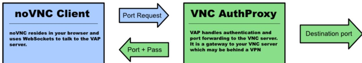
VNCAuthProxy has a control channel that is used to request port forwarding to a specific VNC machine. It will respond with a local port and temporary password that must be used within a short period. This allows a secure connection with the VNCAuthProxy, without compromising the vnc password, and without leaving the port open to anyone with a port scanner.
