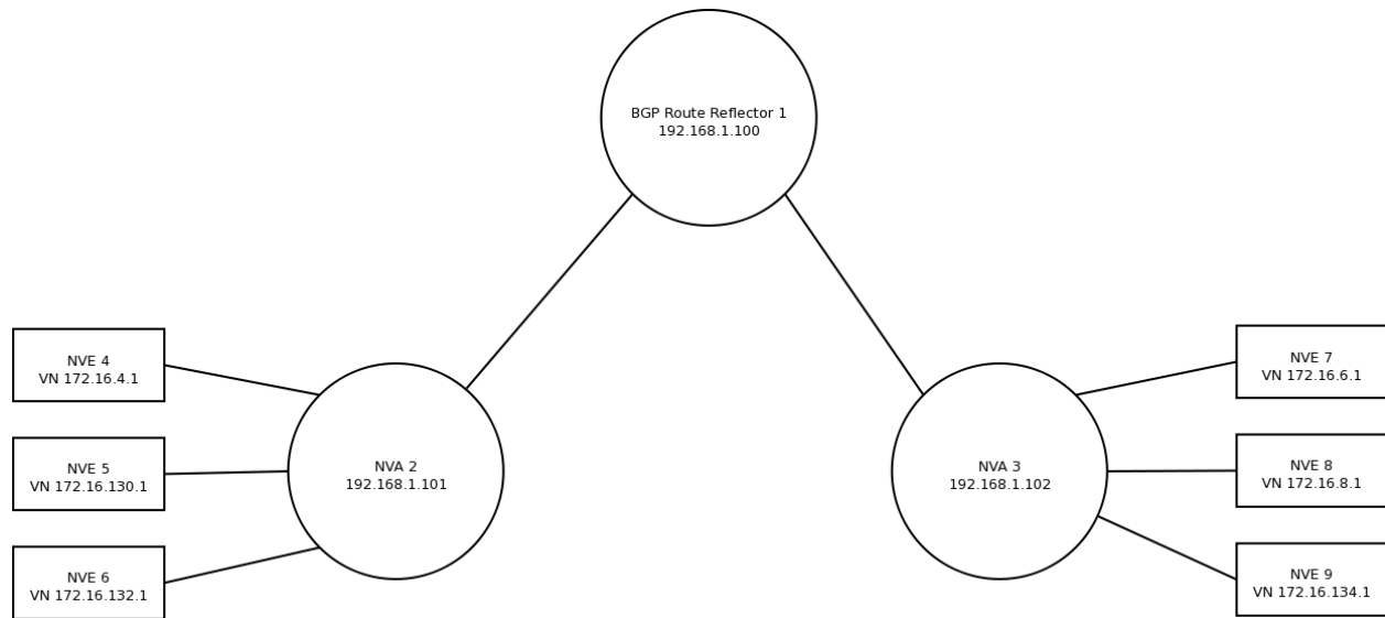
Fig. 7: Two NVAs and a BGP Route Reflector
