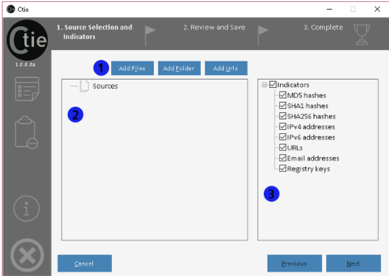
Fig. 3.1: Import one or multiple sources (1). These sources will be displayed in the Sources (2) section and click Next (3) to start the extraction proces.
