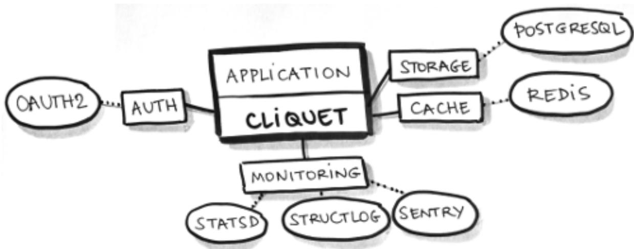
Fig. 2.2: Examples of configuration for a *Cliquet* application in production.
