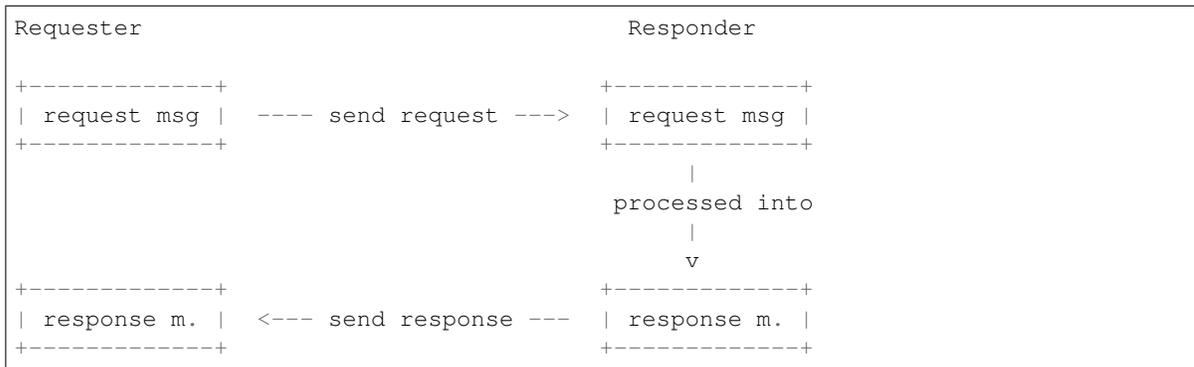
The above shows the four message instances involved in communication between an aiocoap client and server process. Boxes represent instances of Message, and the messages on the same line represent a single CoAP as passed around on the network. Still, they differ in some aspects:
